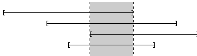
Figure 3.3: For a set S of pairwise intersecting intervals, any point x between the latest starting time and the earliest finishing time (shown shaded) belongs to every interval.
